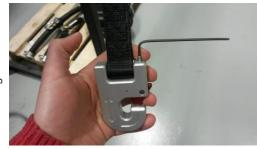
**Step 4)** Ensure the strap can rotate freely about the pin; the assembly is complete. The **Independent Lifter** can now be attached to the ceiling lift.
